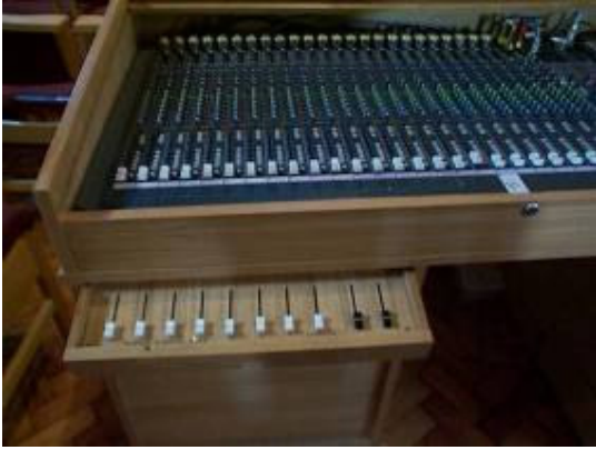
Pull out drawer for simple operation in mixer cabinet
